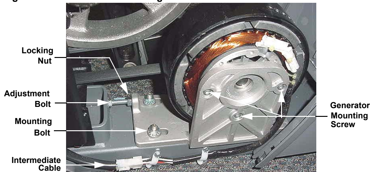
Diagram 7.19 - Generator Mounting
